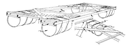
A barge, 8' wide and 20' long, suitable for carrying a float display on water, such as those pictured on this page, can be made with four 50-gallon drums and a wooden framework (III. No. 1).
