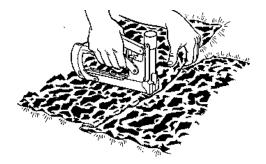
7. Staple the edges down and then staple at random over the entire surface of the foil paper to hold it down securely.
