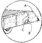
4. To pin sheets together, where the under side is inaccessible to punch pin back through the material with your fingers (such as chicken wire forms, etc.), use an ice pick to guide the pin as shown in illustrations A-B-C-D.
