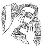
(b) Place bottom of letter along guide line string and press firmly over entire face of letter until it adheres to float
