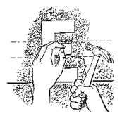
6. To fasten cut-out wallboard letters, place bottom of letter along guide line string and nail to center board of apron
