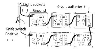
smaller voltages. Use the attachable type reflector made to fit over an ordinary light bulb, with battery powered systems. Use six batteries of 6-volts each connected in series.
