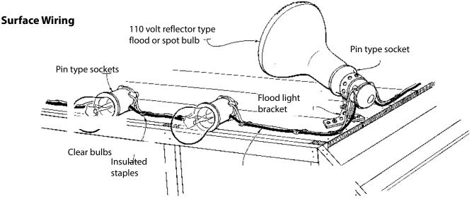
Extreme care should be taken when applying decorating material over surface wiring to prevent driving a staple into the wires. Take extra caution when applying foil paper because it is a good conductor of electricity.
