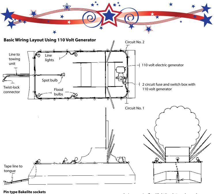
This pin type socket, widely used for float wiring, is easily connected without stripping insulation by placing wires in pin slots and tightening base cap. An inexpensive flood light bracket can be made with perforated pipe strap, a pin type socket, and a ¼" bolt. After mounting, the bracket is easily bent to direct the flood bulb to the desired angle.
