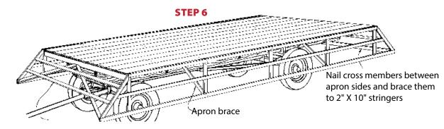
Lower cross member on apron front frame is elevated to allow for trailer tongue clearance
